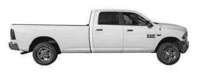
Please be sure to use a pick-up truck with a bed capacity of 3600 lbs minimum and an 8' bed. The bed floor should be approximately 33 3/4" from the ground. The brakes and suspension should be sized appropriately for these loads.
