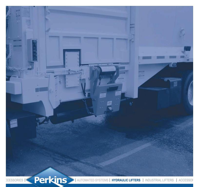
MODEL D6070 SERIES: ROTARY COMPACT LIFTER
