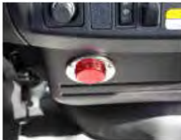
Hoist up in-cab alarm
